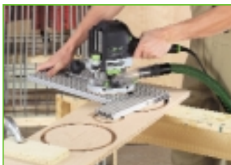
Simple routing of circles: set radius, mount OF 1400 with copying ring.
