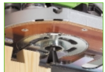
Simply fit it: tool-free change between base runner and copying ring (also available for jointing system VS 600).
